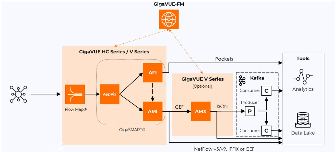
Figure 1 Application Intelligence Solution illustrates how the Application Intelligence solution works.
