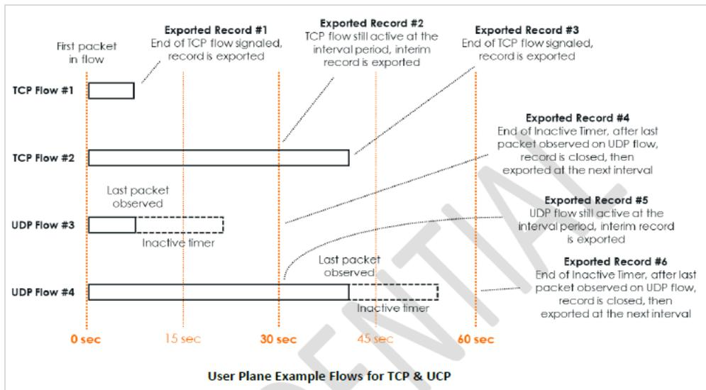
In the diagram above, there are 4 flows, but 6 records are generated. Two flows (#2 & #4) lasted longer than the configured Active Timeout (30 seconds). Therefore, interim records were generated at every 30 seconds. If the flows had lasted longer than 60 seconds, additional interim records would have been generated at 90 seconds, 120 seconds, and so on.
