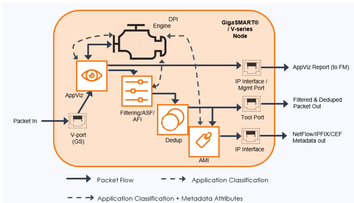
Application Filtering Intelligence (AFI) relies on application classification to filter relevant applications. AFI can be combined with other GigaSMART Operations to further optimize the traffic before forwarding to the tools.
